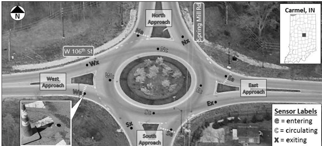
Figure 1: Sensor Layout at the Roundabout at Spring Mill Rd @ W 106th St
