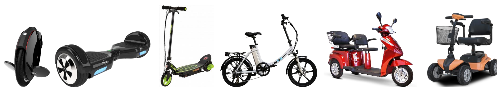
Figure 1 PEMDs – From left electric unicycle, hoverboard, electric scooter, electric bicycle, electric tricycle, and electric mobility cart. (Source: pngkey.com, imgbin.com & iotatrax.com).
